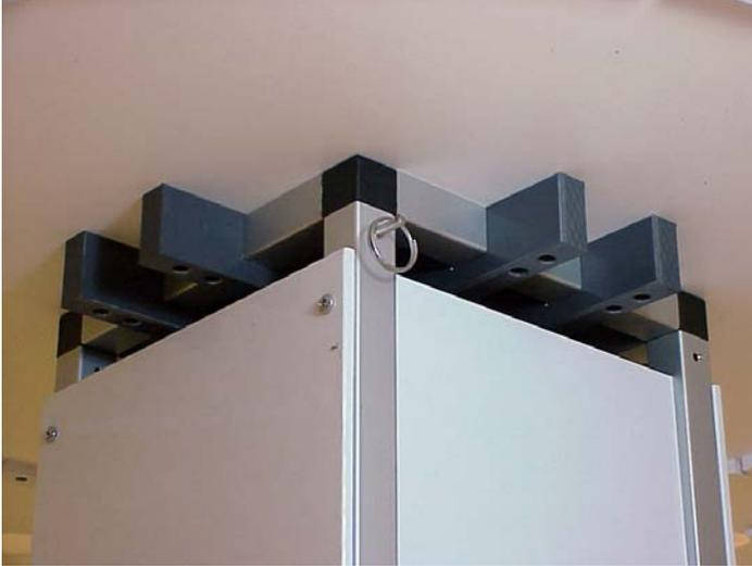
6. Install the goal box by sliding it into the track under the desired hole.
