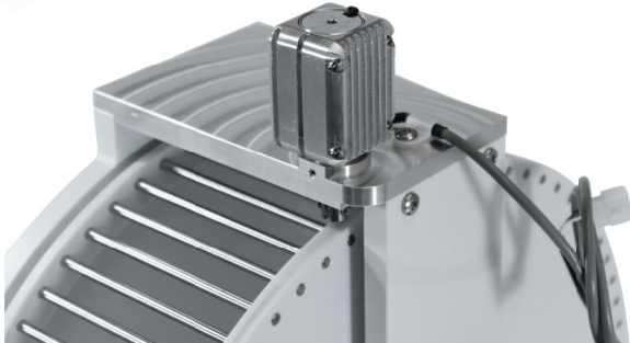
Solenoid Brake Accessory (ENV-042A-SBA) shown on rat activity wheel (ENV-042)
