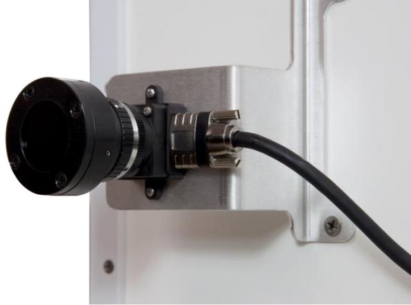
Ensure that the Chamber is pushed all the way to the back of the Cubicle and the NIR light source is turned on in each box. The cameras in the MED-VFC system detect only NIR light; therefore there will be no image on the screen if the NIR light source is off.
